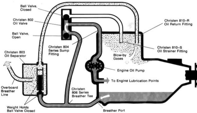
Figure 1, Standard configuration
