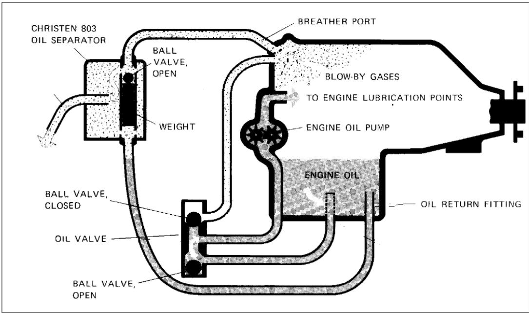
Figure 2, Alternative breather line configuration
